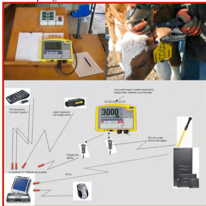
Figure 5. Computer interface for EID and multiple data sampling stations
