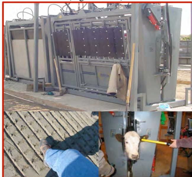
Figure 4. Silencer™ chute, isolation cage, and deep grooving of concrete.
